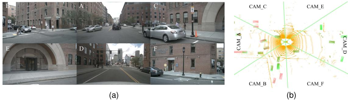
Fig. 13. (a): Image of six cameras deployed around the vehicle, image from nuScenes [43]. (b): BEV view of the 3D detection result, where the red translucent is labeled as ground truth and the green translucent is labeled as the predicted box. The areas corresponding to each of these cameras have been marked on the images.
